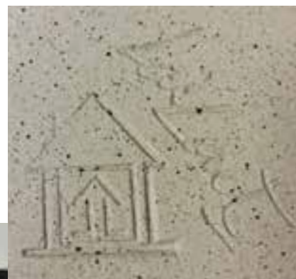
Magnesium die impressions in pottery clay
