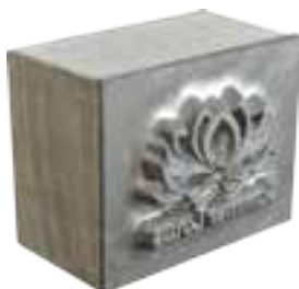
Magnesium die mounted on a wood block
